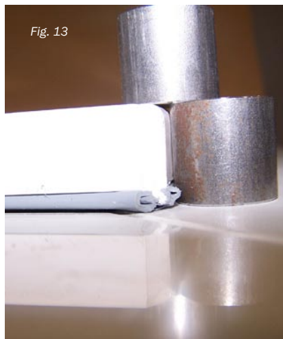
Figure 12: Sealing effect present along the stiles/rails at the end of the test cycle due to rapid elastic recovery in EPDM gaskets
