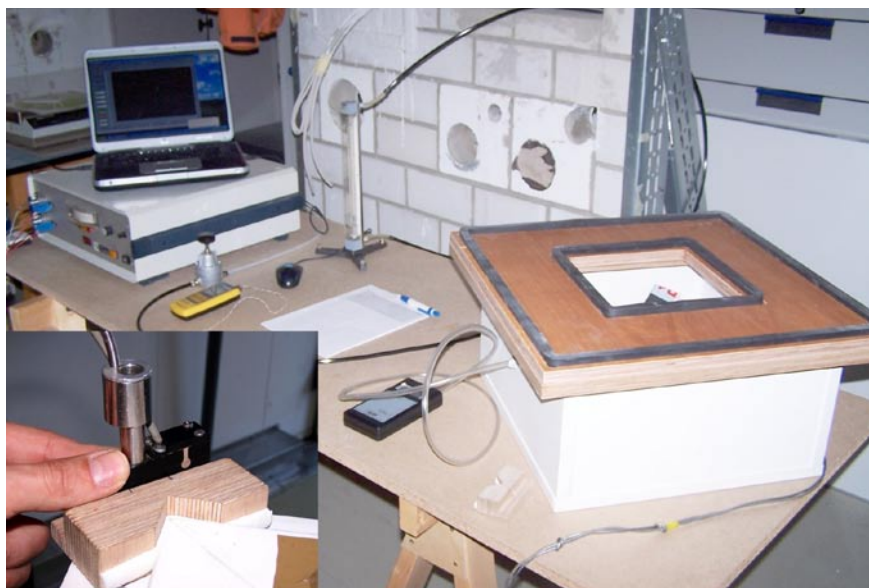
Figure 6: Test set-up and measurement equipment Detail: testing joint perme- ability in the corners
